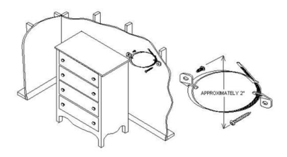
This tip restraint must be attached to a wall stud using the 2" screw enclosed:
